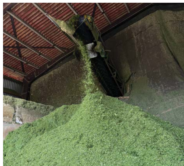
Figure 2 L-R Grass Press-cake and the final feed grade protein from grass which can be fed to cows and pigs respectively (Ausumgaard, Denmark, June 2024).
